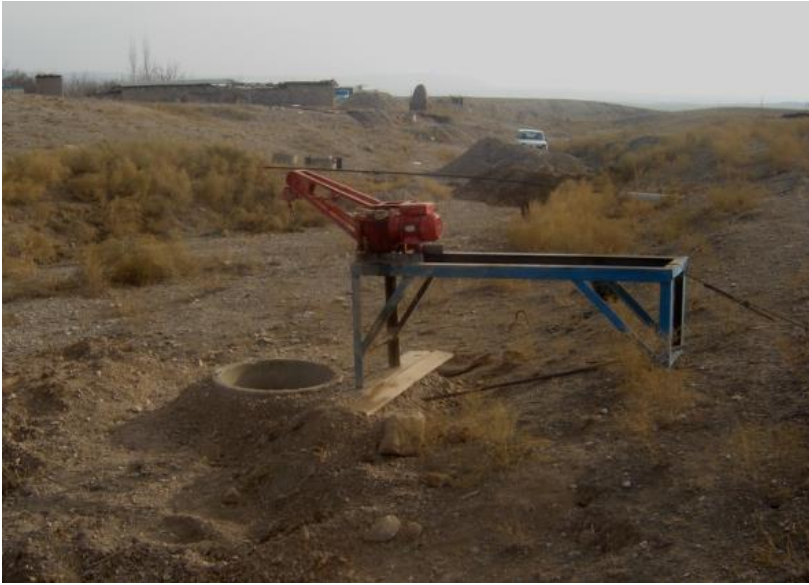
Picture 60. Mobile twist mechanism Lowering and lifting the loads into the ganat bloomery
