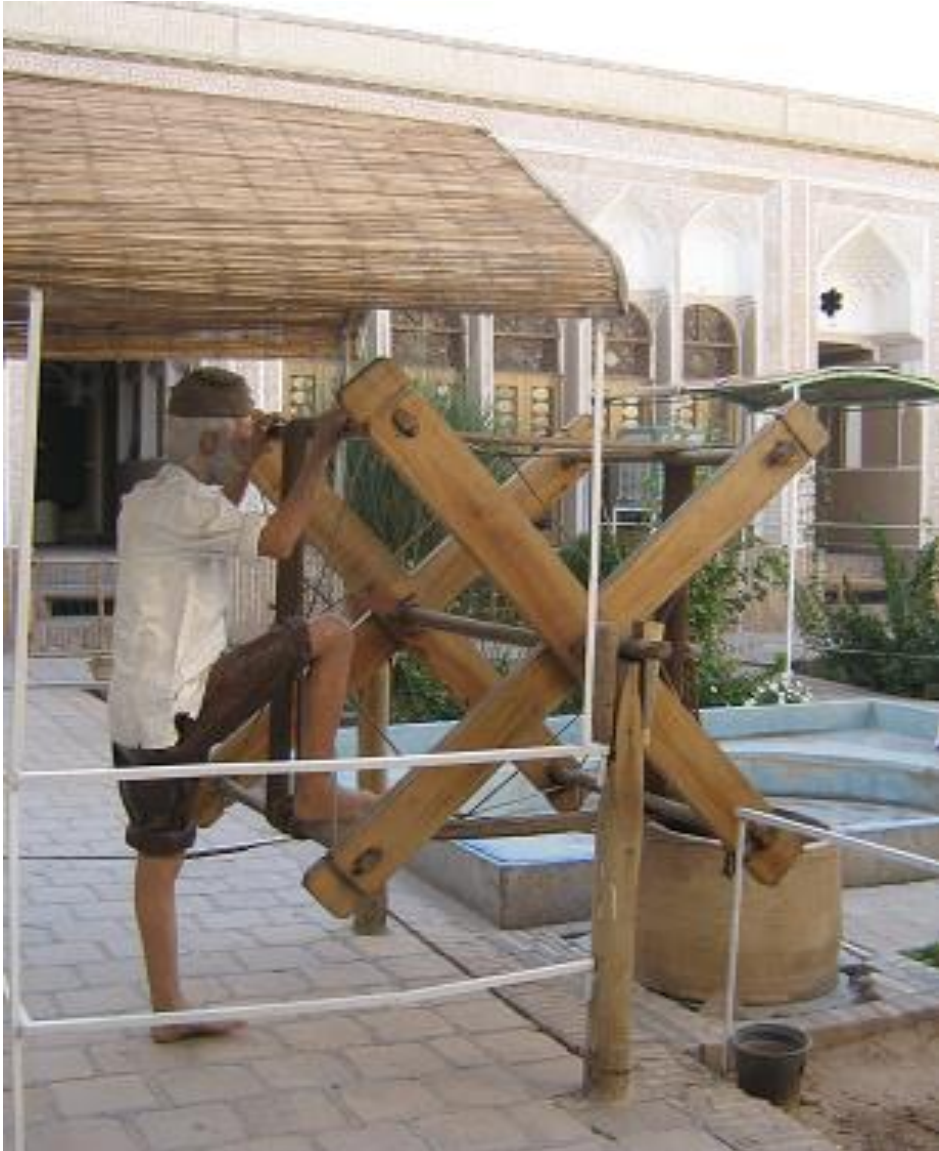
Picture 37. . Kankan wheel and the Kankan working in it. ( Iran Islamic Republic, Yazd Water Museum).
