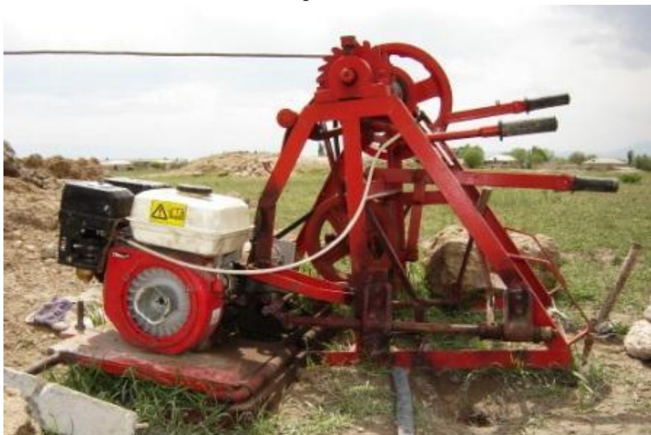
Picture 51. . The loader mechanism with the twist replacing the kankan's wheel
